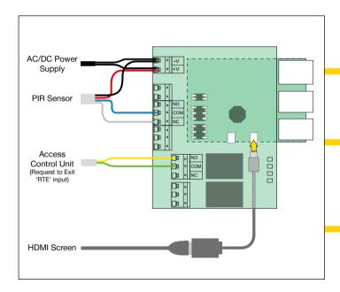
Connections into the Germgard are made by pushing the wire into the terminal block (small wires may need the raised orange part to be pushed down at the same time).
